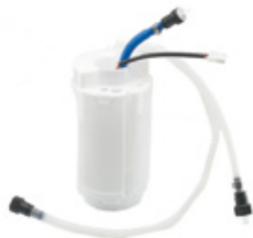
228-236-005-017Z Fuel Supply Unit 1) (FSU) - Fitting Position 2) : Left 4) - Fuel Type 5) : Petrol 6) - Manufacturer Restriction 7) : + Otto - Pressure [bar] 8) : 4
